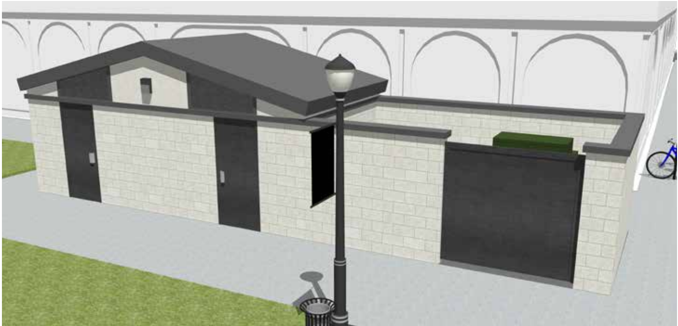
Public restroom shown in design is based on a prefabricated building option for general size and design. Cost estimate assumes build-in-place for financial savings. (Spec below from https://publicrestroomcompany.com/ )
